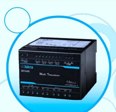
MT440 are intended for measuring and monitoring single-phase or three-phase electrical power network. They measure RMS value by means of fast sampling of voltage and current signals, which makes instruments suitable for acquisition of transient events. A built-in microcontroller calculates measurands (voltage, current, frequency, energy, power, power factor, THD phase angles, etc.) from the measured signals.
